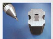
According to different cutting data, wire diameter, angle and workpiece thickness, the AccuteX controller automatically optimize parameters to maintain the best corner cutting performance with high accuracy, as well as cutting speed. Even on the small and continuous corners, accutex still can meet the best corner accuracy.
